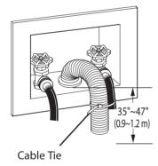
If the water valves and drain are built into the wall, fasten the drain hose to one of the water hoses with the cable tie (ribbed side on inside).
