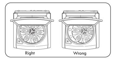
3. To make sure that the washer is properly level, open the lid and look from above to see if the tub is centered. If the tub is NOT centered (as shown in the drawing on the right), readjust the feet. If you have a level, check your washer with the level.
