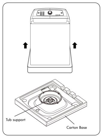
1. After removing the carton and shipping material, lift the washer off the foam base. Make sure the plastic tub support comes off with the base and is not stuck to the bottom of the washer.
