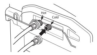
1 Turn OFF both water faucets completely. Unscrew the hot and cold water lines from the back of the washer.
