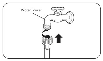
2. Connect the water supply hoses to the HOT and COLD water faucets tightly by hand and then tighten another  $\frac{2}{3}$  turn with pliers.
