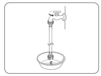
3. Always run a gallon or two of water through each inlet hose to flush dirt, scale and other debris out of the water lines. Doing so will help prevent future problems with clogged filter screens, and will also allow you to verify which hose is hot and which is cold.
