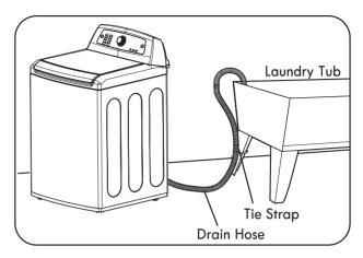
Bend the end of the drain hose to the desired shape and support it on the edge of the laundry tub. Use a tie strap to secure the drain hose in place.
