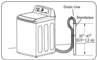
Bend the outlet end of the drain hose to form a U shape. Inset the end of the drain hose into the drain. If the drain is large enough for the flange on the hose to fit inside, then do not insert the flange more than 1-2 inches into the drain. Use the tie strap included with the installation materials in the foam block in the tub to secure the drain hose to the drain.
