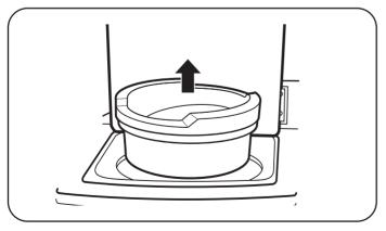
2. Save the foam block for future use. If the washer must be moved in the future, the foam support will help prevent damage to the washer during transportation.
