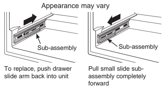
**NOTE:** Make sure the tabs on the full extension drawer guides are fully engaged before loading any bottles. Pull the drawers out all the way to the STOP position and push back in several times to make sure locking tabs are properly engaged.
