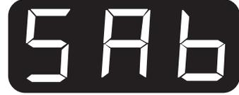
Mode. Controls and lights will not work until the **Red Wine** and **Interior Light** buttons are held again for 7 seconds. The display will show "out" for 1 second and then resume the last operating mode.
